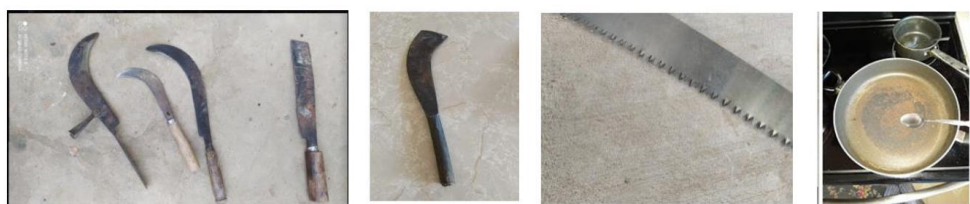
Fig. 6: From the left, (1st inset): A boti used in cutting fish, meat, fruits and vegetables; a small sickle used in cutting fruits, vegetable and light branches of trees; a large sickle used in cutting fish, meat, fruits, vegetables, branches of trees and harvesting crops; and a straight daa used in cutting meat, bamboos, hard branches of trees and dry branches for fuels; (2nd inset): A curved daa with sharp concave side; (3rd inset): A saw with sharp and pointed teeth used in cutting trees and piecing wood; (4th inset): A round rimmed cooking utensil
